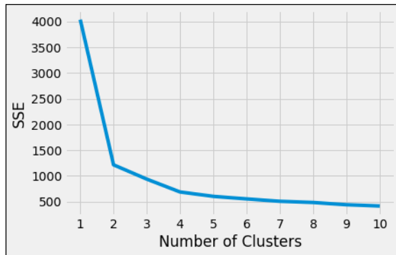
Figure 2: Elbow plot illustrating how the SSE decreases as the number of clusters increases. Note the change in slope at 2 clusters. This indicates that we continue to reduce error as we increase the number of clusters, but at a decreasing rate.
