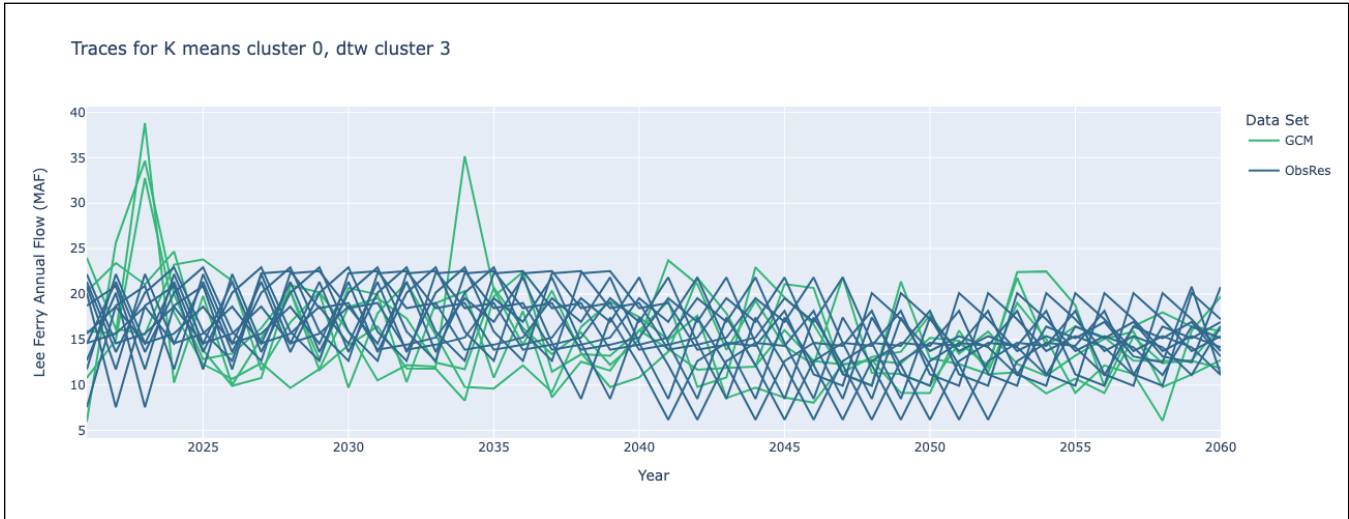
Figure 12: All traces associated with the k means group 0 and dynamic time warping group 3. This represents a cluster of traces that the algorithms placed with one another based on their rolling window/ frequency and duration characteristics and temporal features.
